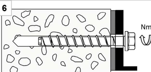
After adjustment, tighten the screw again
