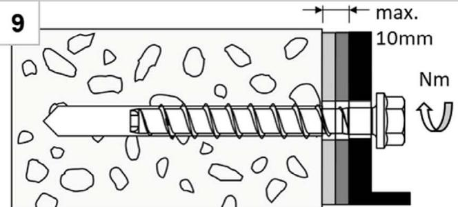
After adjustment, tighten the screw again
