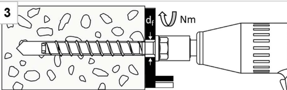
Install with torque impact screw driver or torque wrench
