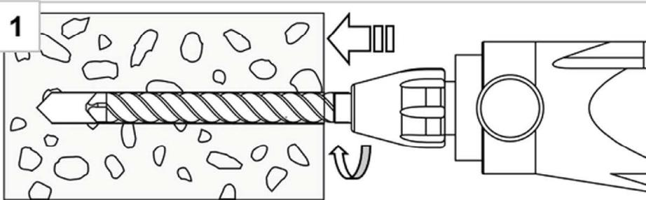
Create hammer drilled or hollow drilled borehole
