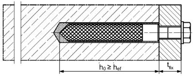
Pre-positioned installation with subsequently injected filling disc (annular gap filled with mortar)
