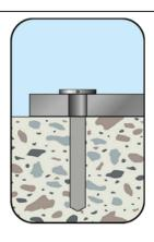
After preparing bore hole (Annex B5), position fixture first, then filling washer
