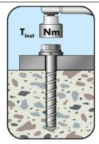
Install with impact screwdriver or torque wrench. Consider  $T_{\text{imp},\text{max}}$  and  $T_{\text{inst}}$
