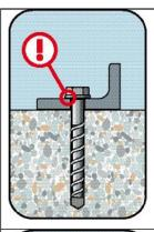
Installation according to **annex B5** until the head of the anchor is fully supported.
