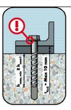
Install the screw again after the adjustment. The total allowed thickness of shims added during the adjustment process is 10mm. The final embedment depth after adjustment process must be equal or larger than  $h_{\text{nom}}$ .
