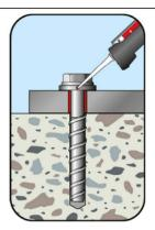
Connect the mixer reduction nozzle to the tip of the mixer. Fill the annular gap with injection mortar. The annular gap is filled with mortar, when mortar oozes out of the washer.
