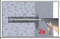
Blow the bore hole clean minimum of 2x with compressed air (min. 6 bar) (Annex B 4) over the entire embedment depth until return air stream is free of noticeable dust. (If necessary, an extension shall be used.)
