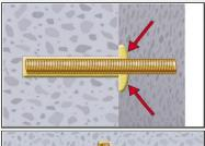
Annular gap between anchor rod and base material must be completely filled with mortar. In case of push through installation the annular gap in the fixture must be filled with mortar also.
