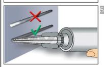
Not proper mixed mortar is not sufficient for fastening. Dispense and discard mortar until an uniform grey or red colour is shown (at least 3 full strokes).
