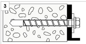
Installed condition without injected mortar in the filling washer
