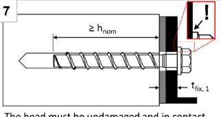
The head must be undamaged and in contact with the fixture
