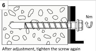
After adjustment, tighten the screw again
