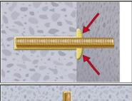
Annular gap between anchor rod and base material must be completely filled with mortar. In case of push through installation the annular gap in the fixture must be filled with mortar also.
