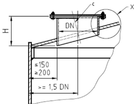
$a \geq 0,7 s_{\min}(\text{WE}) \quad s_{\min}(s_D; s_R)$
