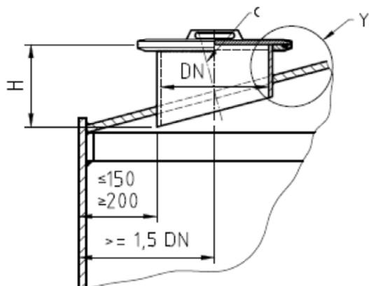
$a \geq 0,7 s_{\min}(\text{WE}) \quad s_{\min}(s_D; s_R)$
