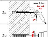
Starting from the bottom or back of the drill hole, blow out the hole with compressed air (min. 6 bar) **four** times, until return air stream is free of noticeable dust.
