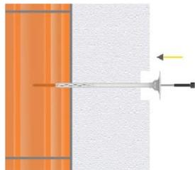
Place the anchor into the drill hole.
