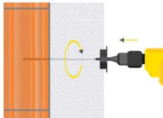
Drill the recess for immersed installation with the tool ZP-FS.
