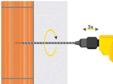
Drill the hole perpendicular to the substrate surface.
