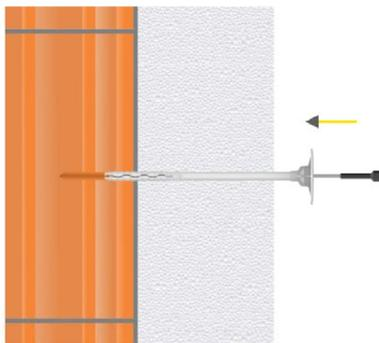
Place the anchor into the drill hole.
