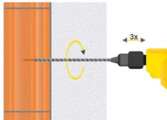
Drill the hole perpendicular to the substrate surface.
