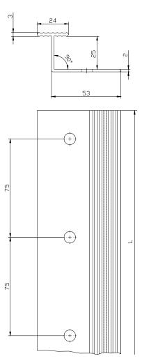
**Vertical connection profile – "PVC Verbindungsleiste"** (dimensions in millimetres)
