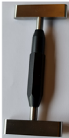
Check of borehole geometry: Length of undercut
