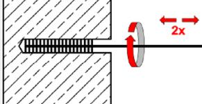
Check brush diameter (Table B4). Brush the hole with an appropriate sized wire brush  $\geq d_{b,min}$  (Table B4) a minimum of **two** times.
