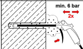
Starting from the bottom or back of the drill hole, blow out the hole with compressed air (min. 6 bar) again a minimum of **two** times until return air stream is free of noticeable dust.
