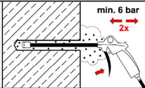
Starting from the bottom or back of the drill hole, blow out the hole with compressed air (min. 6 bar) a minimum of **two** times until return air stream is free of noticeable dust.
