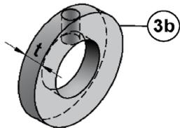
Thickness of washer with bore for diameter
