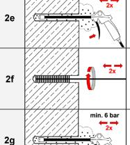
Check brush diameter (Table B4). Brush the hole again with an appropriate sized wire brush  $\geq d_{b,min}$  (Table B4) a minimum of **two** times. If the drillhole ground is not reached with the brush, an appropriate brush
