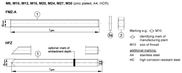
Threaded rod HFT (material sold by the meter, to be cut at the required length) M8, M10, M12, M16, M20, M24, M27, M30 (zinc plated, A2, A4, HCR)
