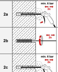
Starting from the bottom or back of the drill hole, blow out the hole with compressed air (min. 6 bar) a minimum of **two** times until return air stream is free of noticeable dust.
