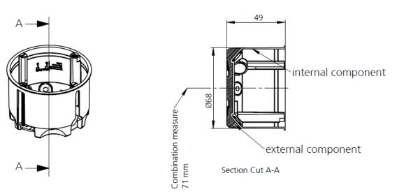
Fire protective one-gang junction box "PROTEC.class PBSDH6862"
