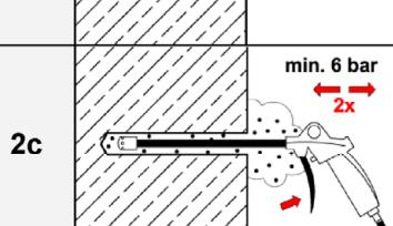
Starting from the bottom or back of the drill hole, blow out the hole with compressed air (min. 6 bar) again a minimum of **two** times until return air stream is free of noticeable dust.
