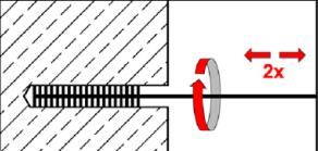
Check brush diameter (Table B4). Brush the hole again with an appropriate sized wire brush  $\geq d_{b,min}$  (Table B4) a minimum of **two** times. If the drillhole ground is not reached with the brush, an appropriate brush extension must be used.
