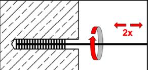
Check brush diameter (Table B4). Brush the hole with an appropriate sized wire brush  $\geq d_{b,min}$  (Table B4) a minimum of **two** times. If the drillhole ground is not reached with the brush, an appropriate brush extension must be used.
