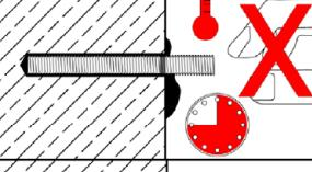
Allow the adhesive to cure to the specified time prior to applying any load or torque. Do not move or load the anchor until it is fully cured (attend Table B6).                                                                                                                                   |
