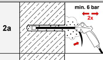
Starting from the bottom or back of the drill hole, blow out the hole with compressed air (min. 6 bar) a minimum of **two** times until return air stream is free of noticeable dust.
