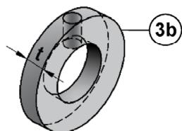
Thickness of filling washer VS
