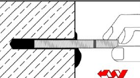
Push the threaded rod or reinforcing bar into the hole while turning slightly to ensure proper distribution of the adhesive until the embedment depth is reached.<br>The anchor shall be free of dirt, grease, oil or other foreign material.                                                      |
