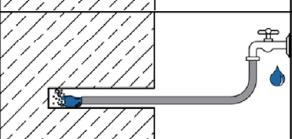
Flush drill hole again with water, starting from the bottom until clear water gets out of the drill hole.
