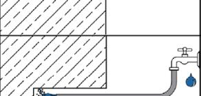
Flush drill hole with water, starting from the bottom until clear water gets out of the drill hole.
