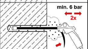
Starting from the bottom or back of the drill hole, blow out the hole with compressed air (min. 6 bar) again a minimum of **two** times until return air stream is free of noticeable dust. If the drillhole ground is not reached, an extension must be used.
