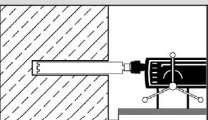
Drill a hole into the base material with prescribed nominal drill hole diameter (Table B1, B2 or B3) and selected drillhole depth. Continue with step 2. In case of aborted drill hole, the drill hole shall be filled with mortar.
