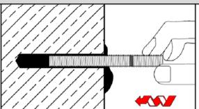
Push the fastening element into the hole while turning slightly to ensure proper distribution of the adhesive until the embedment depth is reached.<br>The anchor shall be free of dirt, grease, oil or other foreign material.                                                                                                             |
