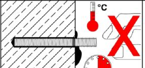
Allow the adhesive to cure to the specified time prior to applying any load or torque.<br>Do not move or load the anchor until it is fully cured (attend Table B6).                                                                                                                                                                         |
