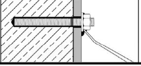
In case of pre-setting installation, the annular gap between anchor rod and fixture may optionally be filled with mortar. Therefore, replace regular washer by filling washer VS and plug on reducing adapter on static mixer.<br>Annular gap is completely filled, when excess mortar seeps out.                                         |
