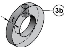
Thickness of filling washer VS
