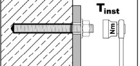
The fixture can be mounted after curing time. Apply installation torque $\leq T_{inst}$ according to Table B1 or B2.                                                                                                                                                                                                                      |
