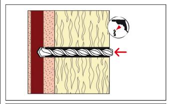
1. Drill hole by corresponding drilling method defined for each stone according to Table C1.1 and drill hole diameter d₀ and depth h₁ according to Table B2.1.
