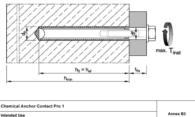
Installation parameters - Internally threaded anchor rod Impact
