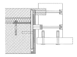
more details according to the technical documentation, horizontal support of the handrail at the top perpendicular to the direction of the walking line
