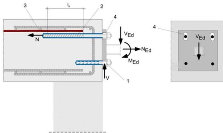
The required transverse reinforcement acc. to EN 1992-1-1:2011 is not shown in the figures. **The fischer rebar anchor may be only used for axial tensile force.** The tensile force must be transferred by lap to the existing reinforcement of the building. The transfer of the shear force has to be ensured by suitable measure, e.g. by means of shear force or anchors with European Technical Assessment (ETA).
