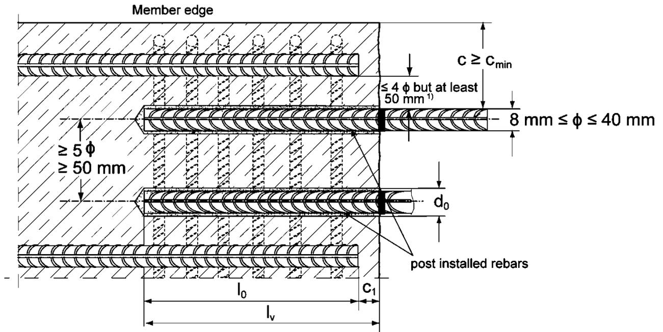
1) If the clear distance between lapped bars exceeds  $4\phi$  but at least 50 mm then the lap length shall be increased by the difference between the clear bar distance and  $4\phi$  but at least 50 mm.
