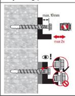
A screw can be adjusted maximum two times. The total allowed thickness of shims added during the adjustment process is 10 mm. The final embedment depth after adjustment process must be larger or equal than  $h_{\text{nom2}}$  or  $h_{\text{nom3}}$ .
