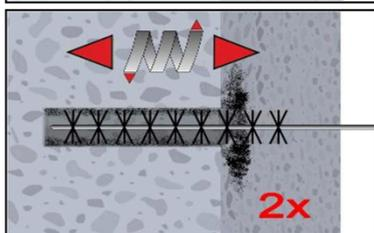
2e. Brush the bore hole minimum 2x with brush RB according to Table B3 over the entire embedment depth in a twisting motion. (If necessary, a brush extension RBL shall be used.)
