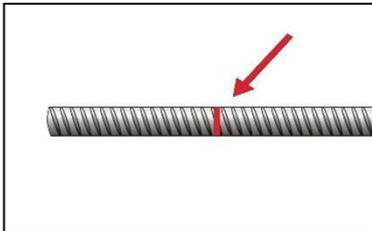
4. Mark embedment length  $l_b$  on the reinforcing bar .
