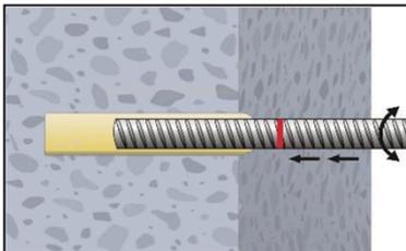
**9.** Insert the reinforcing bar while turning slightly up to the embedment mark.
