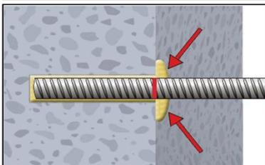
**10.** Annular gap between reinforcing bar and base material must be completely filled with mortar. Otherwise, the installation must be repeated starting from step 8 before the maximum working time  $t_{work}$  has expired.
