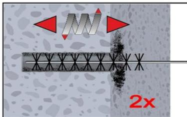
2b. Brush the bore hole minimum 2x with brush RB according to Table B3 over the entire embedment depth in a twisting motion. (If necessary, a brush extension RBL shall be used.)
