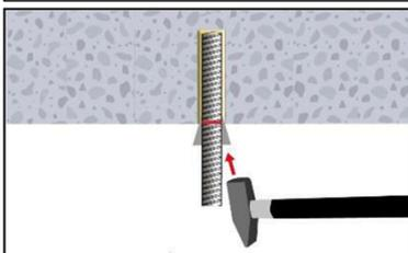
**11.** For application in vertical upwards direction the reinforcing bar shall be fixed (e.g. wedges).
