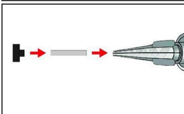
7. Piston plugs VS and mixer nozzle extensions VL shall be used according to Table B3 or B4.
