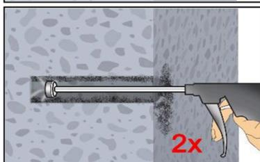
2f. Finally blow the bore hole clean minimum 2x with compressed air (min. 6 bar, oil-free) (Annex B 4) over the entire embedment depth until return air stream is free of noticeable dust. (If necessary, an extension shall be used.)
