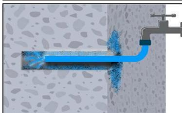
2c. Flushing again with water until clear water comes out.
