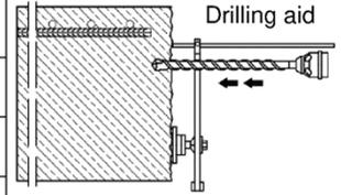
Comments: The minimum concrete cover acc. EN 1992-1-1:2004+AC:2010 must be observed.
