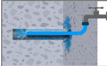
2a. Flushing with water until clear water comes out.
