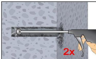
2d. Blow the bore hole clean minimum 2x with compressed air (min. 6 bar, oil-free) (Annex B 4) over the entire embedment depth until return air stream is free of noticeable dust. (If necessary, an extension shall be used.)
