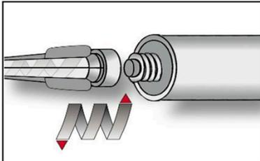
3. Screw on static-mixing nozzle PM-19E, and load the cartridge into an appropriate dispensing tool.
