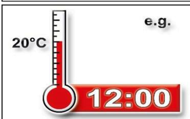
**12.** Temperature related curing time  $t_{cure}$  (Annex B 4) must be observed. After initial curing time  $t_{cure,ini}$  has elapsed, the installation of the connecting reinforcement and the formwork can be continued. The full load to the reinforcing bar may be applied after the full curing time  $t_{cure}$  has elapsed.
