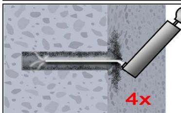
2c. Finally blow the bore hole clean minimum 4x from the bottom or back by hand pump (Annex B 4).
