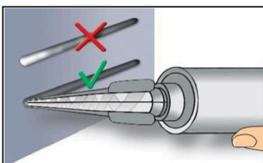
6. Not proper mixed mortar is not sufficient for fastening.
