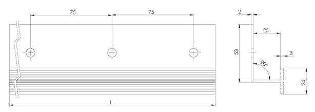
Vertical connection profile - "Sto-Verbindungsleiste PVC" (dimensions in millimetres)
