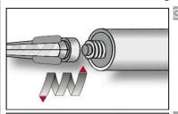
Screw on static-mixing nozzle CRW 14W/PM-19E and load the cartridge into an appropriate dispensing tool. With foil tube cartridges cut off the foil tube clip before use.
