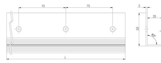
Vertical connection profile - "Verbindungsleiste PVC" (dimensions in millimetres)
