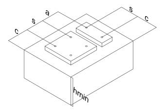
Fixing points with a spacing a  $\leq$  s<sub>cr,N</sub> are considered as a group with a maximum characteristic resistance N<sub>Rk,p</sub> according to Table 17. For a spacing a > s<sub>cr,N</sub> the anchors are considered as single anchors, each with a characteristic resistance N<sub>Rk,p</sub> according to Table 17.
