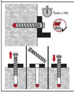
After minimum curing time of 24 h the HUS4 screw can screw out and in for 1 time.
