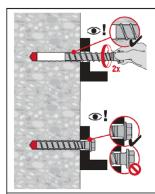
Find the thread in the drilled hole
