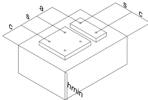
Fixing points with a spacing  $a \leq s_{cr,N}$  are considered as a group with a maximum characteristic resistance  $N_{Rk,p}$  according to Table 17. For a spacing  $a > s_{cr,N}$  the anchors are considered as single anchors, each with a characteristic resistance  $N_{Rk,p}$  according to Table 17.
