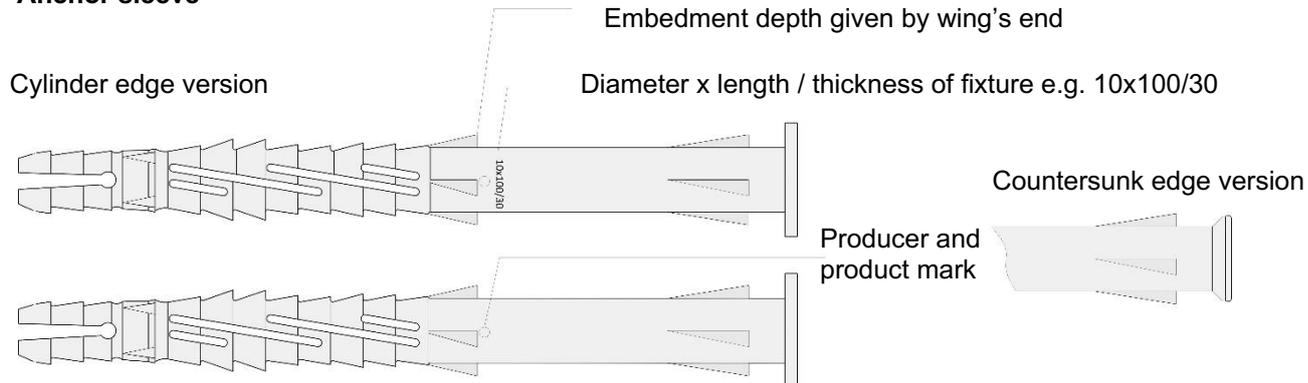
**Special screw (Carbon steel version and stainless steel A4 version)**
