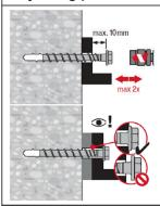
A screw can be adjusted maximum two times. The total allowed thickness of shims added during the adjustment process is 10 mm. The final embedment depth after adjustment process must be larger or equal than the required one of  $h_{nom1}$ ,  $h_{nom2}$  or  $h_{nom3}$ .
