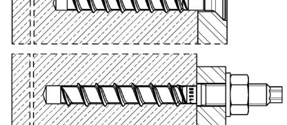
HUS4-A (threaded rod connection sizes 10 with M12 and 14 with M16)
