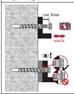
A screw can be adjusted maximum two times. The total allowed thickness of shims added during the adjustment process is 10 mm. The final embedment depth after adjustment process must be larger or equal than  $h_{\text{nom}}$ .
