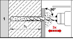
When the drill hole depth ( $h_1$ =  $h_{ef}$  +31mm) is reached, move the drill back and forth at least three times with the machine switched on to remove the dust in the drill hole (venting the drill hole). Continue with step 3.
