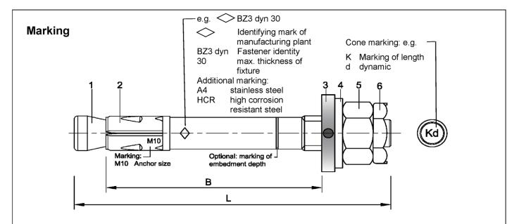
Usable length:  $B = h_{ef} + t_{fix}$
