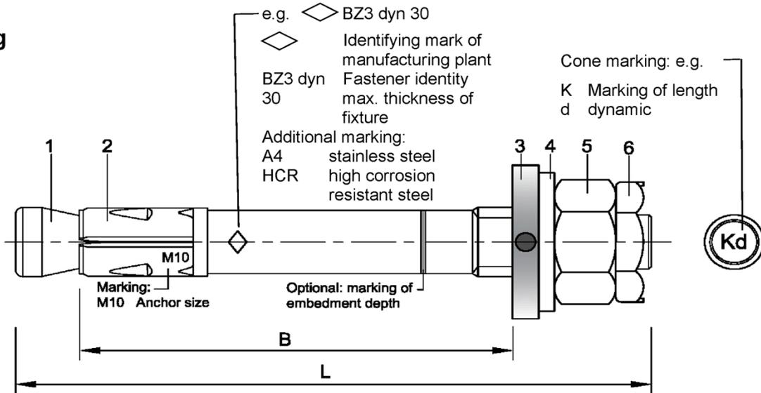
**Usable length:**  $B = h_{ef} + t_{fix}$
