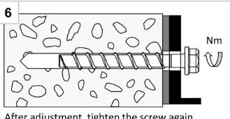
After adjustment, tighten the screw again
