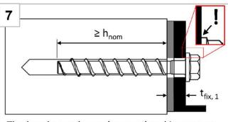
The head must be undamaged and in contact with the fixture
