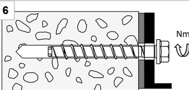
After adjustment, tighten the screw again
