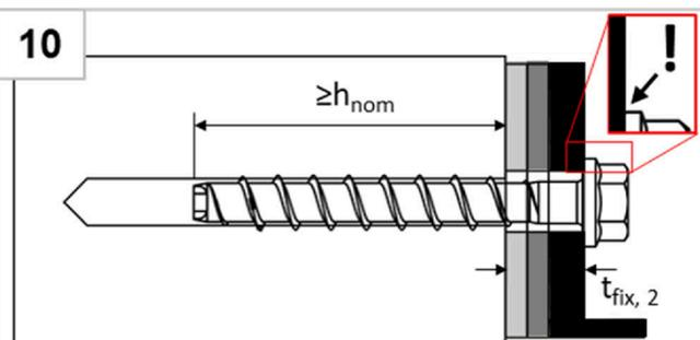
The head must be undamaged and in contact with the fixture
