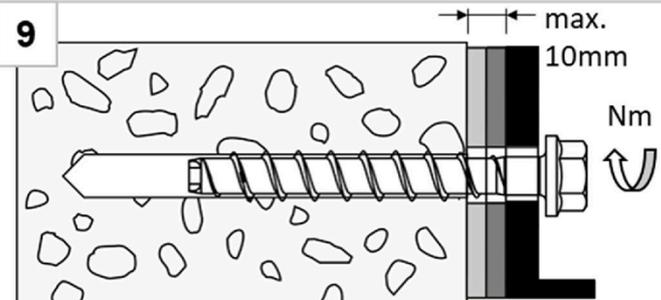
After adjustment, tighten the screw again
