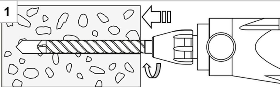
Create hammer drilled or hollow drilled borehole
