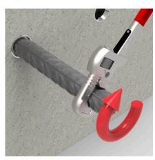
Use a standard wrench to tighten the rebar. For rebar with  $\emptyset \ge 25$  mm, use a minimum lever length of 0,80 m.
