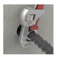
Set the rebar in the correct position and use a standard wrench to tighten the lock nut. For rebar with  $\emptyset \ge 25$  mm, use a minimum lever length of 0,80 m.
