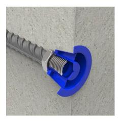
No visible threads on the rebar outside the lock nut; the spacing plug (RFI) is properly installed.
