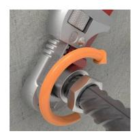
Use a standard wrench to tighten the coupler. For rebar with  $\varnothing \ge 25$  mm, use a minimum lever length of 0,80 m
