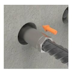
The lock nut is fully engaged on the  $2^{nd}$  phase rebar; coupler and lock nut are in contact.
