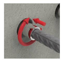
Approach the 2nd Phase Rebar to the 1st Phase Rebar until they are in contact, then start rotating the coupler.
