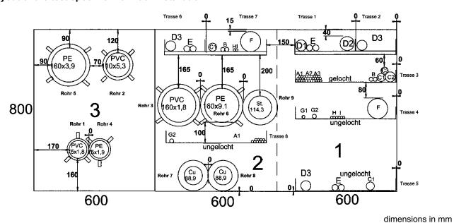
Use as part of a mixed penetration seal with a resistance to fire class **EI 90**Layout of the test specimens in wall and floor – front view
