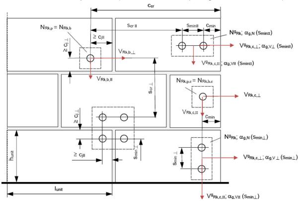
c<sub>min</sub> = minimum edge distance to the free edge of the wall
