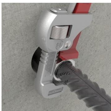
Set the rebar in the correct position and use a standard wrench to tighten the lock nut. For rebar with  $\varnothing \geq 25$  mm, use a minimum lever length of 0,80 m.
