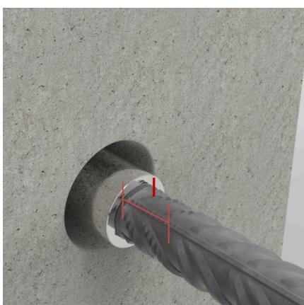
When the installation is completed, the visible threading length "l" has to fall between the limits below indicated.
