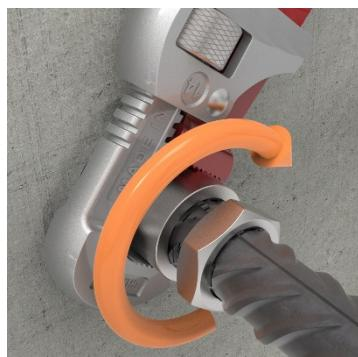
Use a standard wrench to tighten the coupler. For rebar with  $\varnothing \geq 25$  mm, use a minimum lever length of 0,80 m
