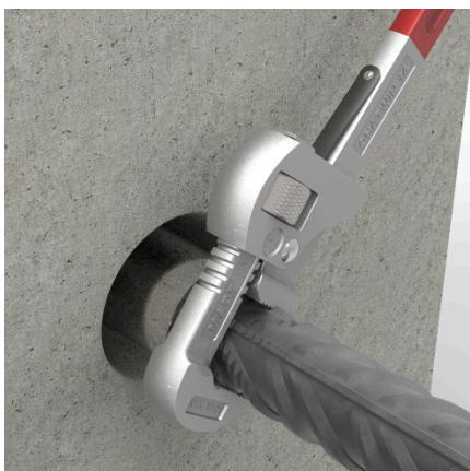
Use a standard wrench to tighten the rebar. For rebar with  $\varnothing \geq 25$  mm, use a minimum lever length of 0,80 m
