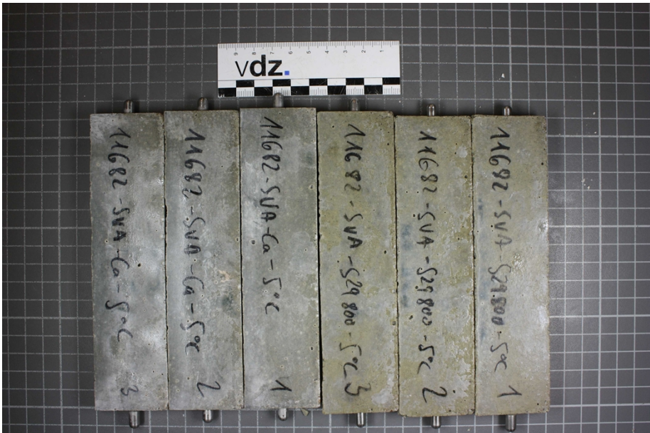
Figure A2: Specimens with CEM III/A 52,5 N-SR "Rotterdam" after 180 days; Storage: 5 °C in \text{Ca}(\text{OH})_2 -solution (3 left-hand side specimens) and in \text{Na}_2\text{SO}_4 -solution (3 right-hand side specimens)
