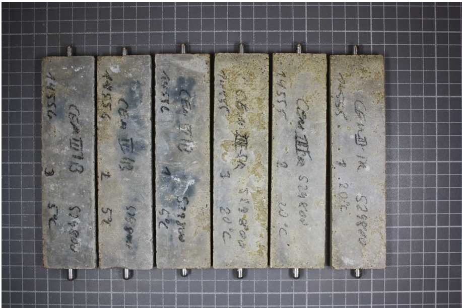
Figure A3: Specimens with CEM III/B 42,5 N-LH/SR after 180 days; Storage: in Na 2 SO 4 -solution at 5 °C (3 left-hand side specimens) and at 20 °C (3 right-hand side specimens)
