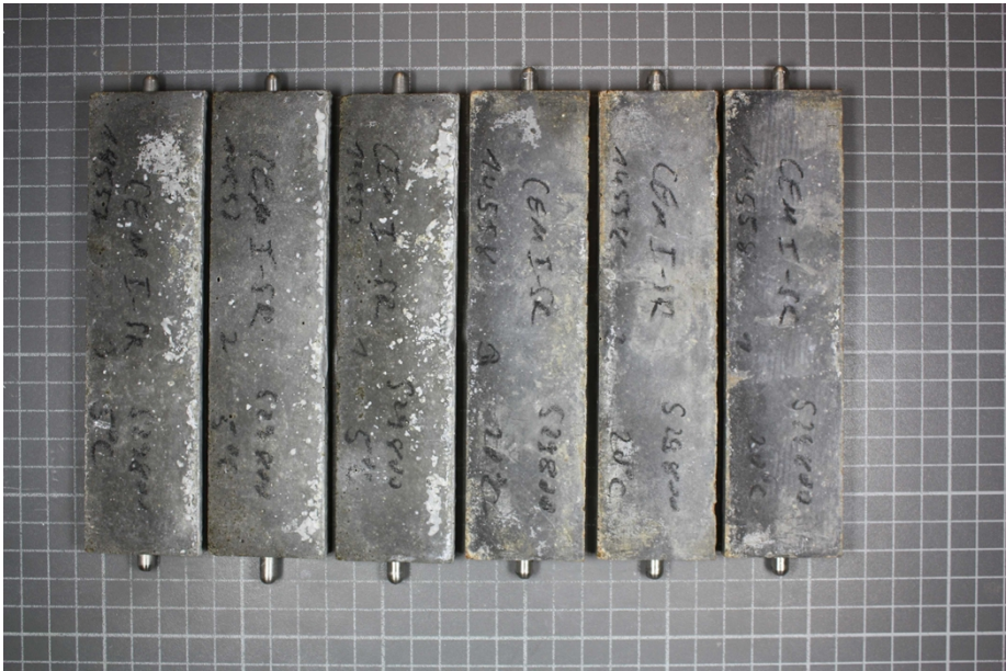
Figure A4: Specimens with CEM I 42,5 R-SR3 after 180 days; Storage: in Na 2 SO 4 -solution at 5 °C (3 left-hand side specimens) and at 20 °C (3 right-hand side specimens)
