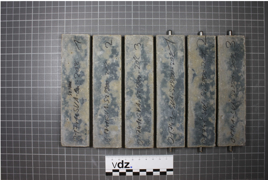
Figure 5: Specimens with CEM III/A 52,5 N-SR/LA (C2 with blast furnace slag 2 (S2)) after 180 days; storage: 20 °C in Na 2 SO 4 solution
