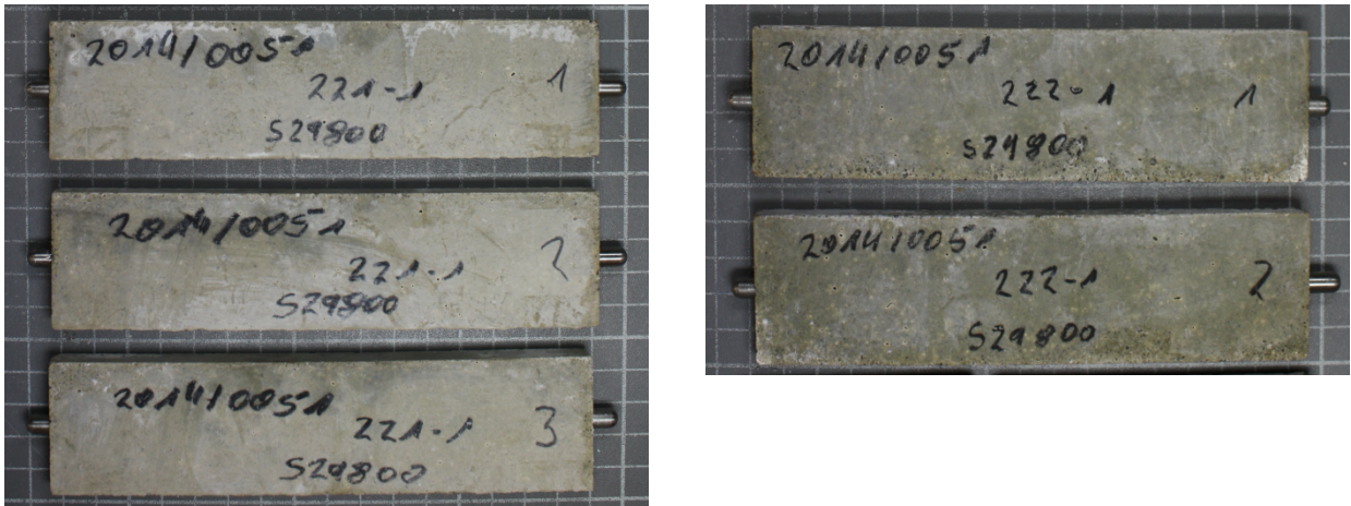
Figure 3: Specimens with CEM III/B 42,5 N-LH/SR after 180 days; storage: in Na 2 SO 4 solution at 20 °C (on the left) and at 5 °C (on the right)
