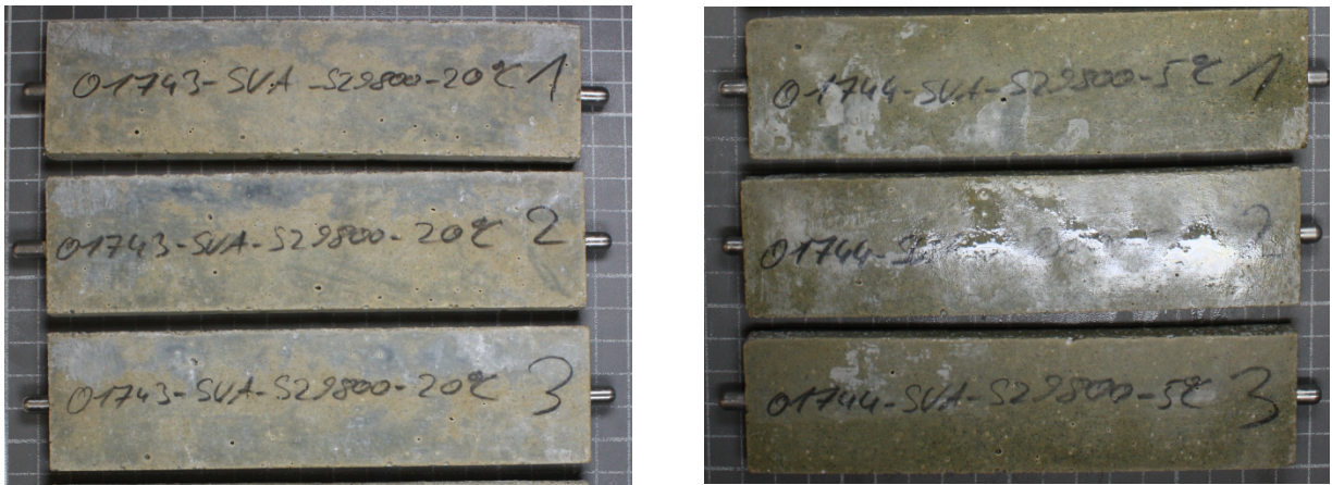
Figure 7: Specimens with CEM III/B 42,5 N-LH/SR after 180 days; storage: in Na 2 SO 4 solution at 20 °C (on the left) and at 5 °C (on the right)
