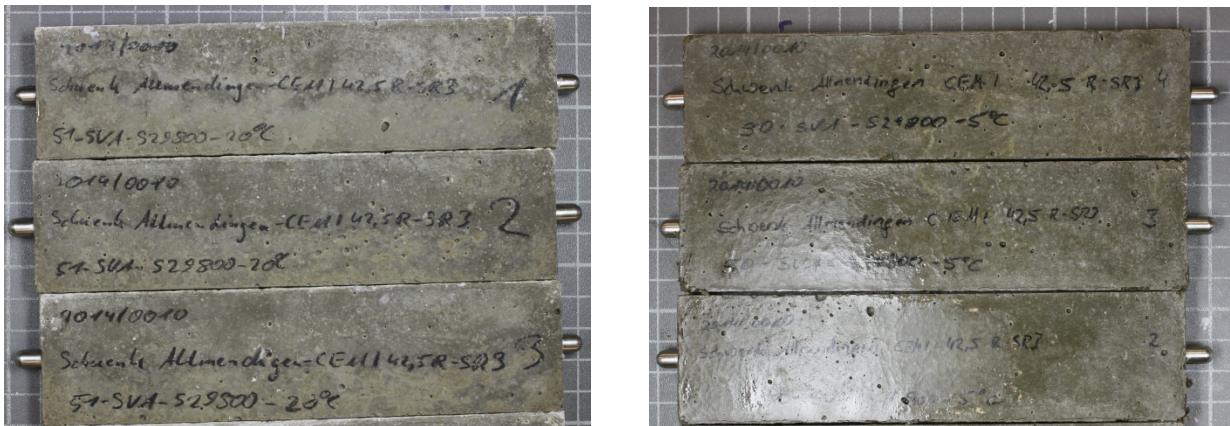
Figure 8: Specimens with CEM I 42,5 R-SR3 after 180 days; storage: in Na 2 SO 4 solution at 20 °C (on the left) and at 5 °C (on the right)
