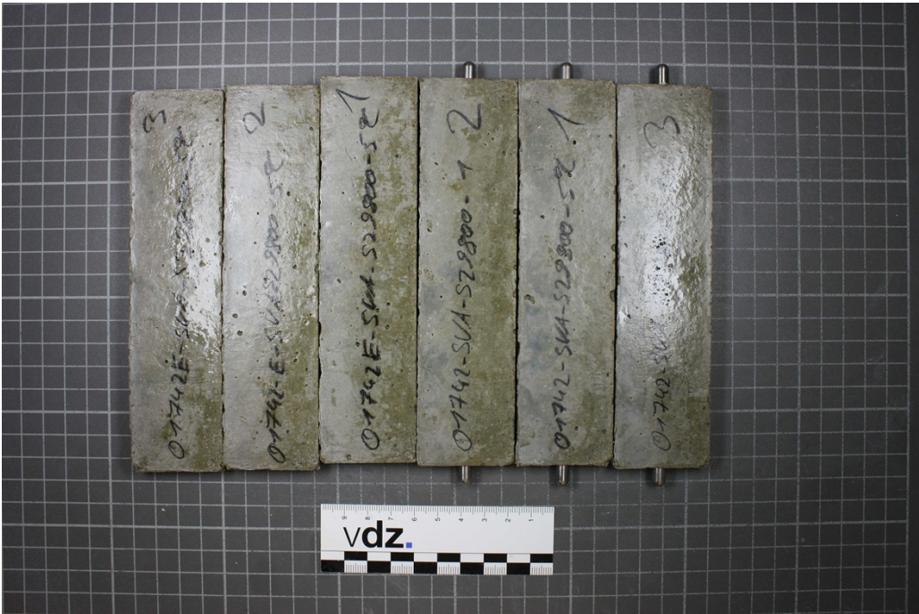
Figure 6: Specimens with CEM III/A 52,5 N-SR/LA (C2 with blast furnace slag 2 (S2)) after 180 days; storage: 5 °C in Na 2 SO 4 solution
