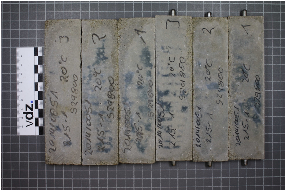
Figure 1: Specimens with CEM III/A 52,5 N-SR/LA (C1 with blast furnace slag 1 (S1)) after 180 days; storage: 20 °C in Na_2SO_4 solution
