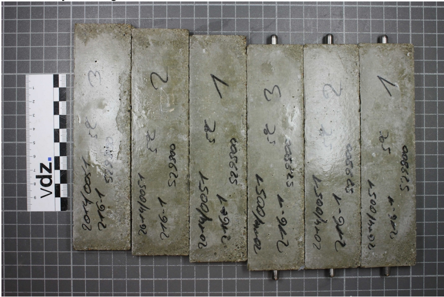
Figure 2: Specimens with CEM III/A 52,5 N-SR/LA (C1 with blast furnace slag 1 (S1)) after 180 days; storage: 5 °C in Na_2SO_4 solution
