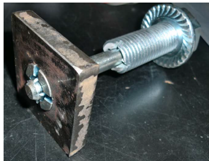
Figure 2: Installed Molabolt after tensile testing
