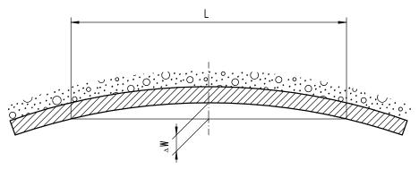
Figure 2 - Deformations of backing plates.
