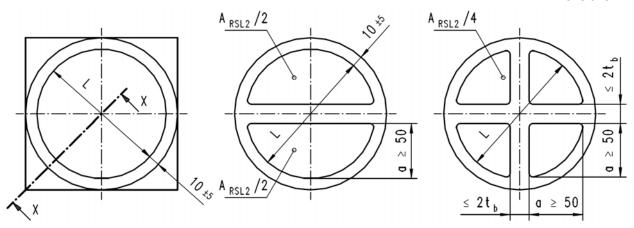
Figure B.2 - Examples of recessed flat ROBO®SLIDE L2 configurations
