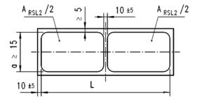
Figure B.4 - Examples of recessed ROBO®SLIDE L2 sheets for guides
