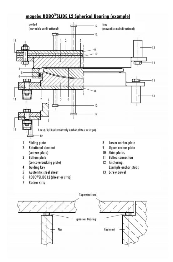
Figure A.1 - Assembly of a guided and free movable spherical bearing with mageba ROBO®SLIDE L2 and its intended use (example)
