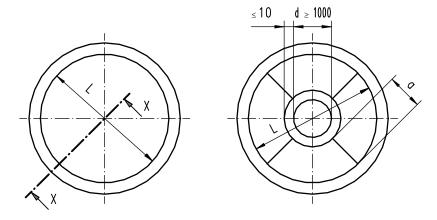
Figure B.3 - Subdivision of recessed ROBO®SLIDE L2 sheets for spherical sliding surfaces
